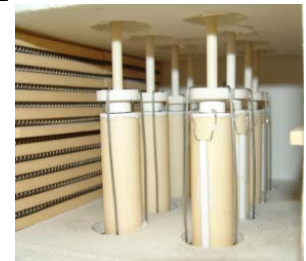
Multiple button cells in furnace, each with individual gas flow and electrical controls
